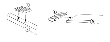
**Step 8**: Place the Slats (9) into hardware part (E) then press hardware part (F) firmly into the Side Supports (5) **DO NOT use any power tools as this may damage the frame and will invalidate any claim.**
