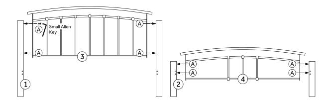
**Step 2**: Fix the Side Support (5) to the Headposts (1) and Footposts (2) using hardware parts (A). Do not fully secure the screws yet before Step 6.
